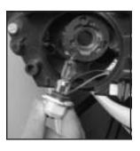
Remove the bulb from the bulb socket.
